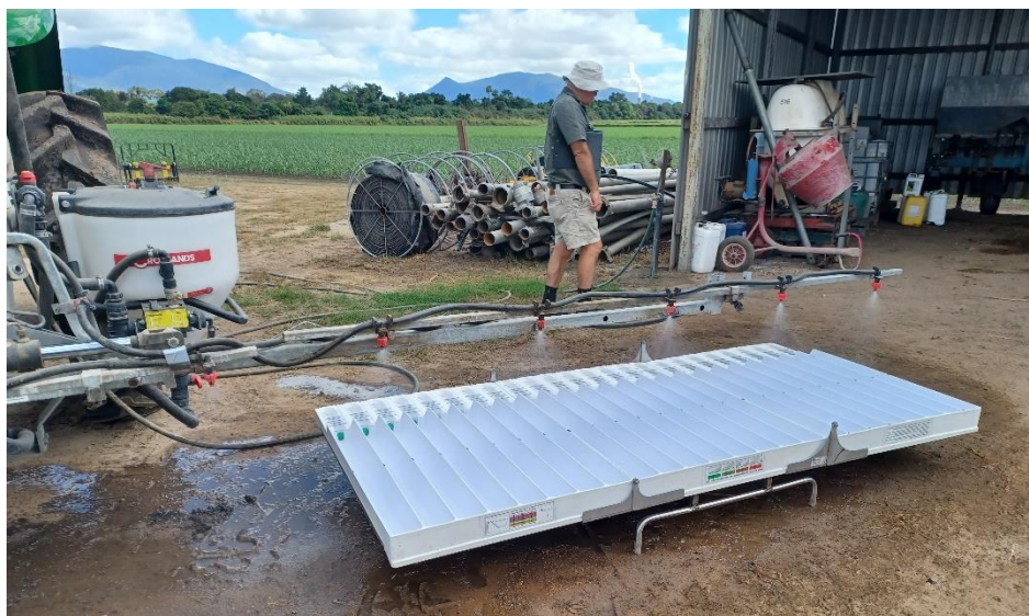
Figure 1: Patternator under spray boom catching droplets
