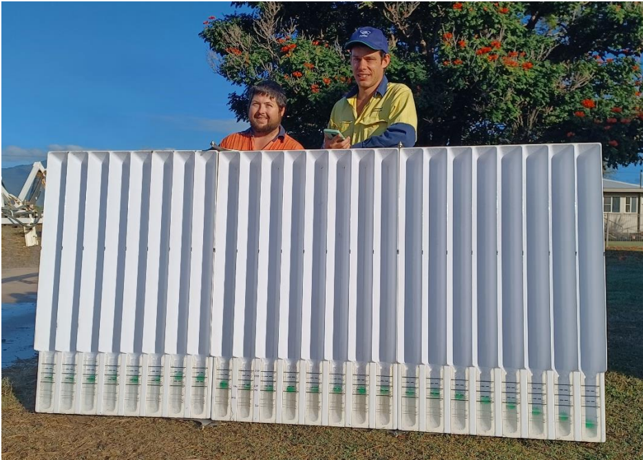
Figure 2: spray rig distribution displayed by the patternator, notice the height of the balls taper towards the edges.
