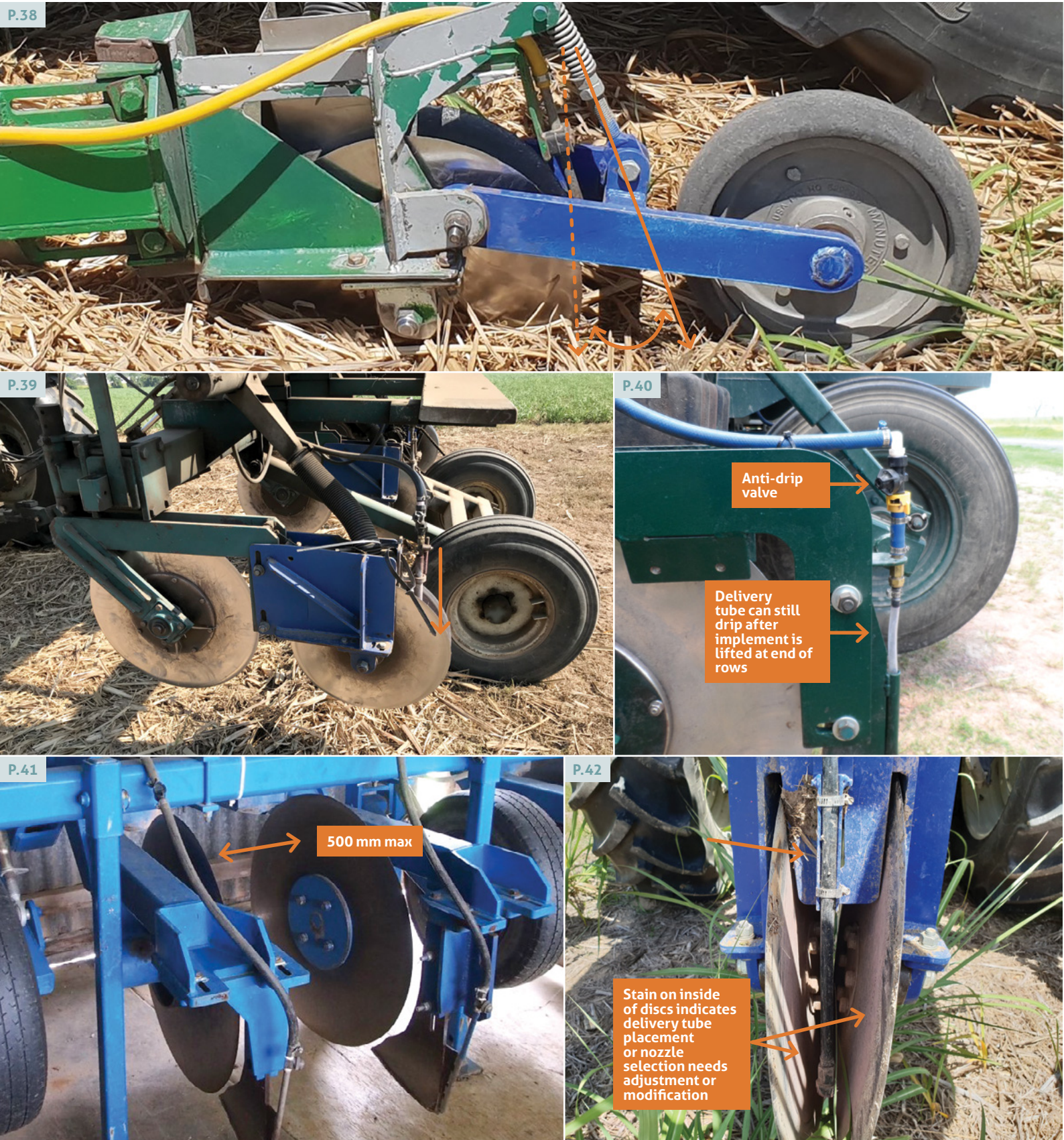
Photo 38 - The nozzle on this applicator is angled too far back, resulting in shallow application and wetting of the press wheel. It is easily rectified by adjusting the angle forward. The solid arrow shows the existing nozzle angle and the dashed arrow shows the correct nozzle angle. Photo 39 - Correct alignment of nozzle ensuring liquid reaches the base of the slot. However, this applicator could be improved by the addition of a slot closure mechanism. Photo 40 - Coulter/tyne applicator showing the anti-drip valve, and the protective metal tubing to house the delivery tube. This applicator could also be improved with the addition of a slot closure mechanism. Photo 41 - A twin coulter applicator - the horizontal distance between the coulters must be 500 mm maximum. Photo 42 - Scraper fitted to double disc to minimize buildup of wet fertilizer granules on inner surfaces. This applicator also could be improved with the addition of a slot closure mechanism and by directing the imidacloprid stream away from the discs so that the liquid does not contact them.
