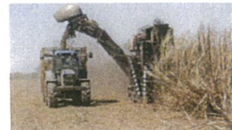
Measuring cane yield with commercial harvesters and weighing equipment. Sucrose content (CCS) is analysed by Near Infrared Spectroscopy (NIR).
