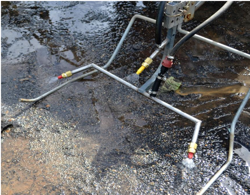
Figure 2: Dual herbicide spray bar. Glyphosate is applied through the centre Nozzle and other herbicide mixes applied through the 2 wing nozzles
